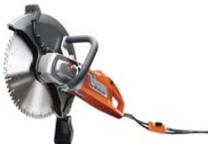
This electric disc cutter offers wet and dry cutting in one machine. Unlike petrol-driven cutters it emits no fumes and so is ideal for work in tight, confined spaces. An optional vac unit allows for easy transformation into a dry cutter that produces minimal dust. The blade rotates forwards to offer efficient cutting with minimal user effort.
